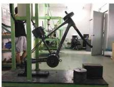
3. Pedaling fatigue test 踩踏疲劳测试
