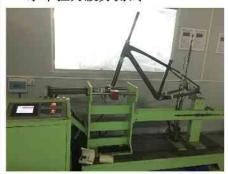
5. Vertical fatigue test 垂直拉力疲劳测试
