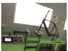
3. Pedaling fatigue test 踩踏疲劳测试
