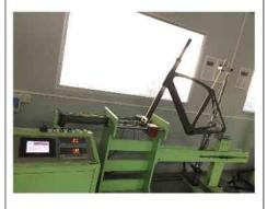
2. Impact test (Falling frame) 车架前倒冲击测试
