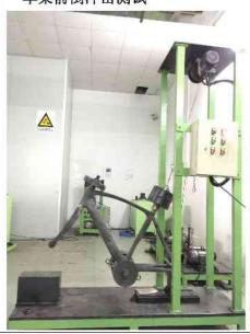
5. Vertical fatigue test 垂直拉力疲劳测试
