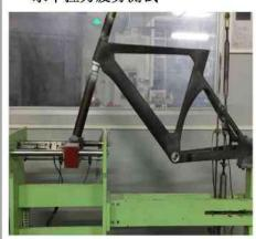
2. Impact test (Falling frame) 车架前倒冲击测试
