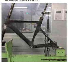
3. Pedaling fatigue test 踩踏疲劳测试
