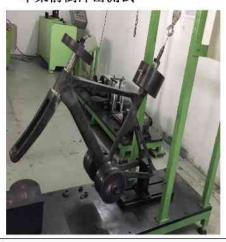
5. Vertical fatigue test 垂直拉力疲劳测试
